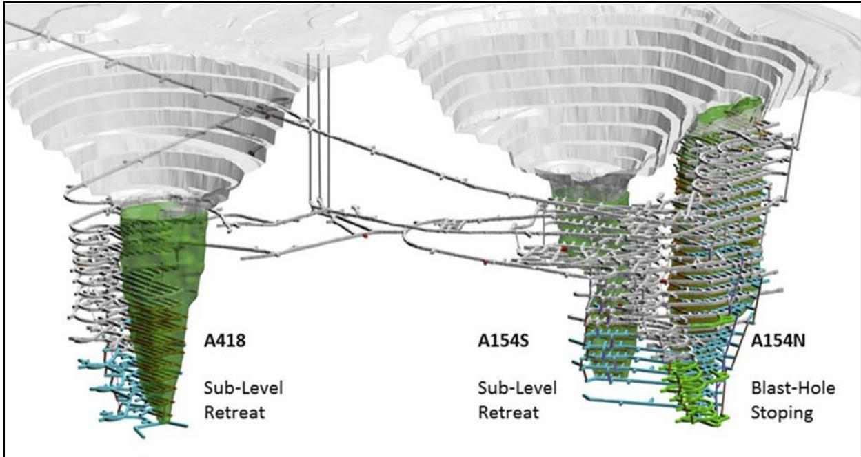
Figure 4: Diavik underground mining at A418 and A154
