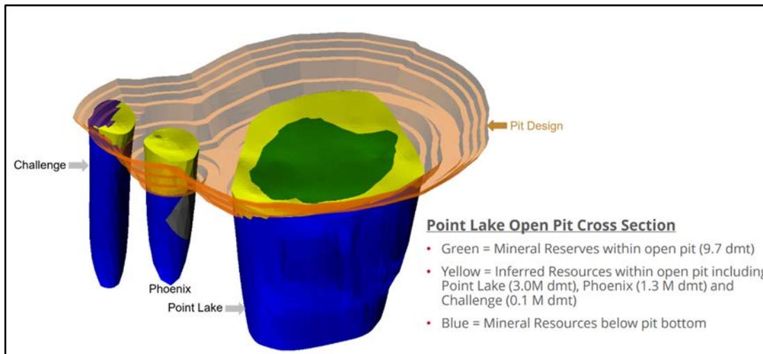
Figure 7: Point Lake open pit with Point Lake, Phoenix and Challenge pipes
