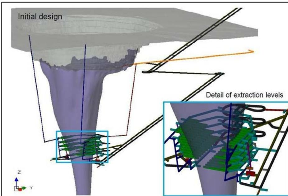
Figure 9: Conceptual layout inclined cave mining of Fox underground
