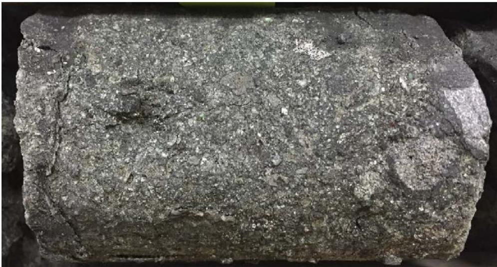
Figure 26: Drill core from mud-rich to olivine rich RVK (KIMB2)
