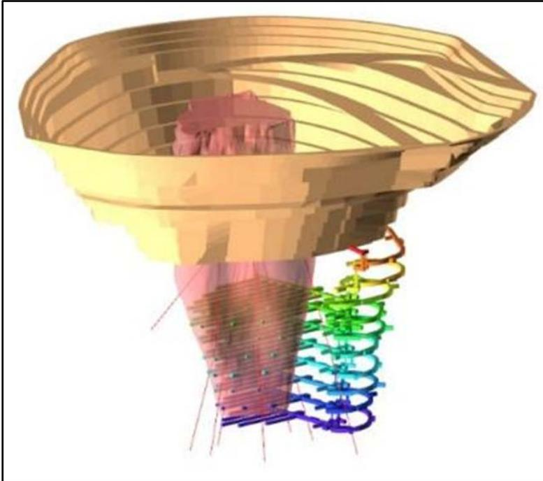
Figure 8: Preliminary mine design for Sable underground (sublevel retreat)
