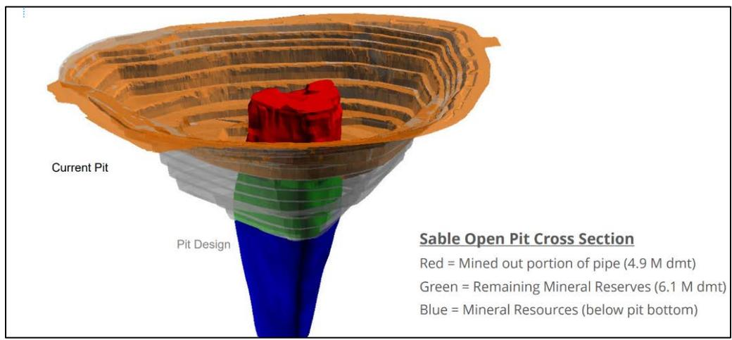
Figure 5: Sable open pit mineral reserves as of Dec 31st 2022
